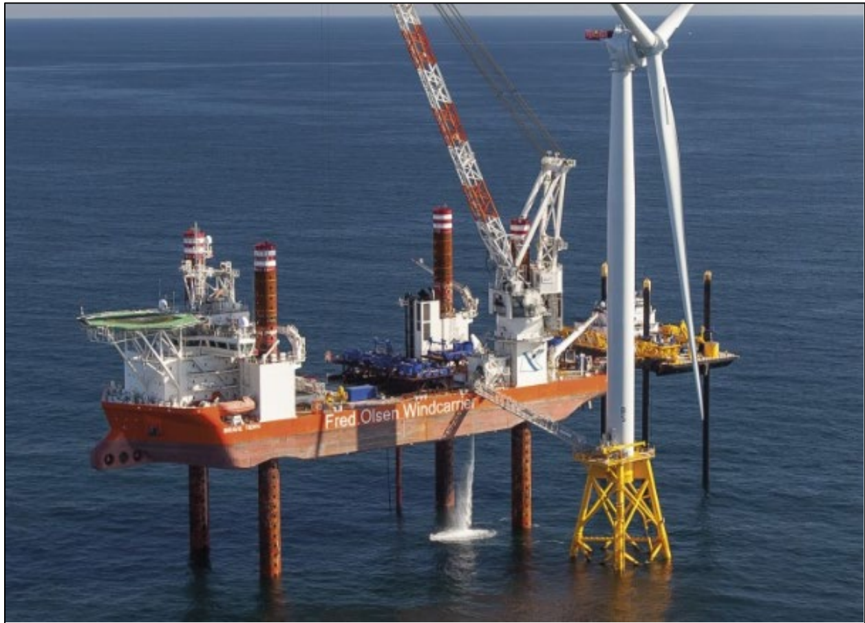
Figure 10.10 WTG Installation Vessel and feeder jack-up barge at Work - Installation of a WTG Blade (Block Island, 2016)
