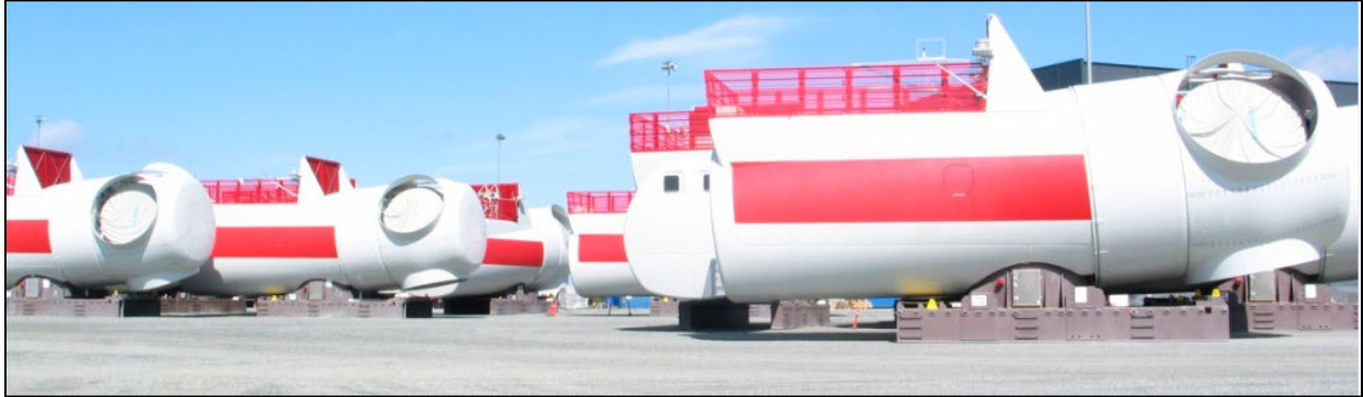
Figure 10.7 Nacelles Pre-assembled and Ready at the Load Out Port (Gode Wind, 2015)
